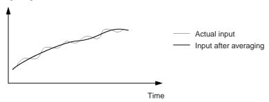
**Note** The time required for converted data refreshing remains 2 ms/point when the averaging function is enabled. The first communications data after the power is turned ON will be output after averaging eight samples.
