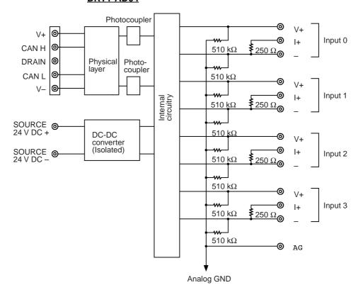
**Note** The DRT1-AD04H has insulation between the inputs, so there is no need for the user to be concerned with the internal circuitry.
