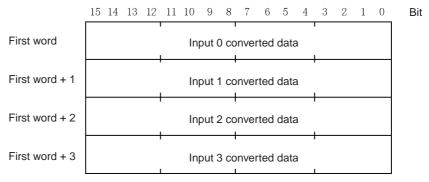
If the converted data is a negative number, it is expressed as a two's complement. The NEG command can be useful to obtain the absolute value from the two's complement.
