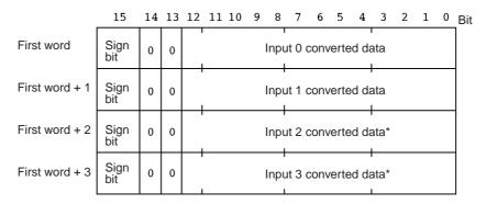
**Note** \*Not used when there are two input points. At that time only two words are occupied.
